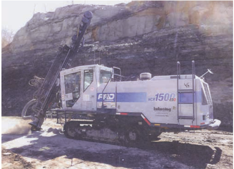
The Furukawa 1500 Pre-Split Drill provided by Kokosing for a class held in Martin County, KY
